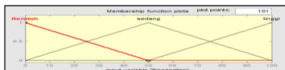
Figure 2. Speed variable membership function input
