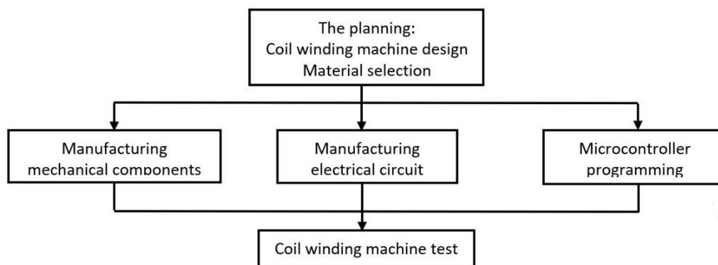
Figure 1. Stages of coil winding machine design
