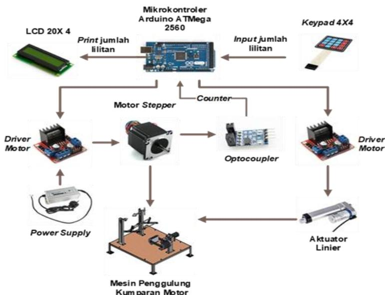
Figure 3. Schematic control of an electric motor coil winder machine
