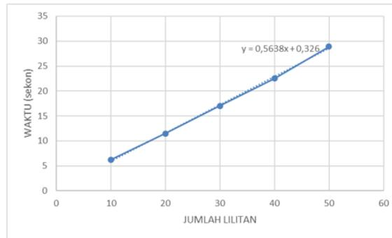
Figure 4. Graph of results of winding speed testing
