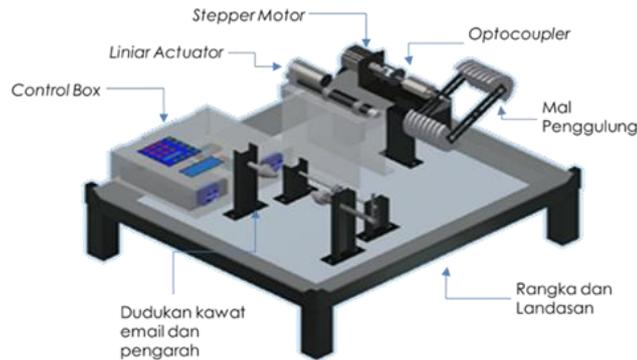
Figure 2. Optimization of coil winding machine design
